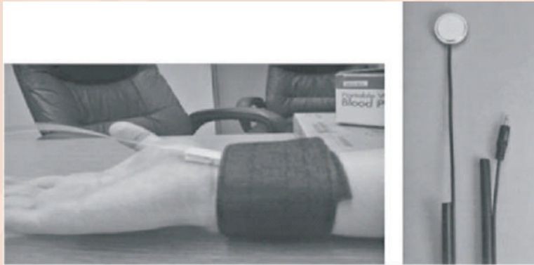
Figure 2 (a) Piezoelectric blood pressure monitor fixed on the wrist. Courtesy: Wade D. Peterson, David A. Skramsted, and Daniel E. Glumac, Reproduced from the website: www.phoenix.tc-ieee.org . (b) Pro-Wave's piezoelectric blood pressure sensor. Courtesy: Pro-Wave Electronic Corp.
